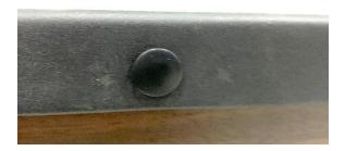
Through the exterior access, reinstall fasteners removed earlier which are located at brackets to the front and rear. Retorque these fasteners to 27 N-M (20 ft lb)
