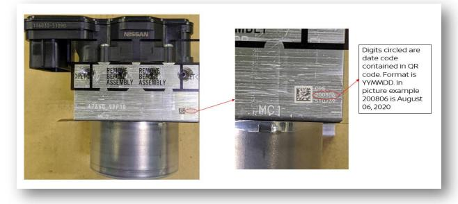
Alternatively, if the date code is damaged or illegible, a QR Code Reader application may be downloaded to a smartphone and used to scan the QR code to identify the manufacture date of the part.
