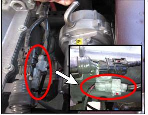
10. Disconnect the brake vacuum pump electrical connector.
