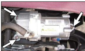
12. Remove three 12 mm bolts to disconnect the brake vacuum pump assembly.
