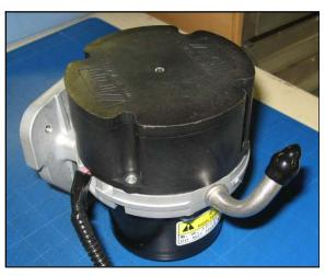
14. Replace the brake vacuum pump with the new unit.
