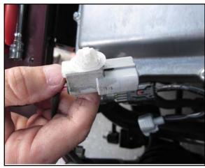
11. Unclip the brake vacuum pump electrical connector mount from the vehicle's body.
