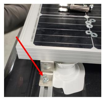
9. Insert bolt through the rear leg of the solar panel. Install the washer and locking nut. Tighten with an 11mm nut socket.
