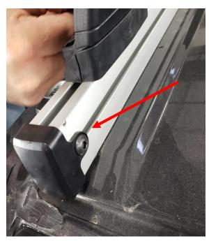
1. Using Allen wrench remove black cap from track (keep screw in a safe place to reuse).
