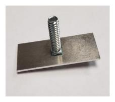
4. From parts kit, insert carriage bolt into plate hole; repeat for 3 other plates.
