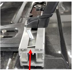
5. Slide plate and carriage bolt (x2) into track channel. Lift luggage bar to slide both sets of plates and bolts down the track channel. Slide luggage rack bar bolt and plate back in place and secure bar to track with washer and nut. Tighten.
