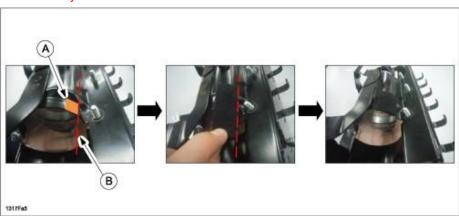
b. Attach the other felt tape on the other side of the retainer.
