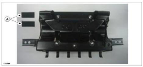
a. Attach one piece of felt tape in the straight area of the retainer (A) using the red line (B) on the lower part of the straight edge as reference. Fold in half and paste inside the retainer.
