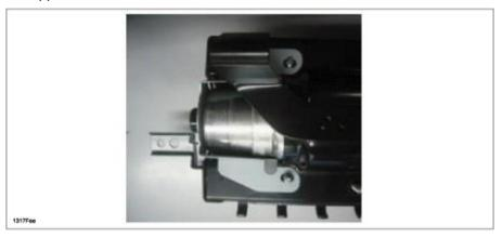
9. Install the new M5 nuts and one used nut (in position 3) as shown, then tighten the 5 nuts to the specified torque in the order shown.
