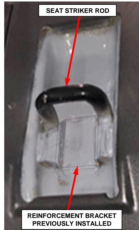
Figure 17 – Reinforcement Bracket Previously Installed
