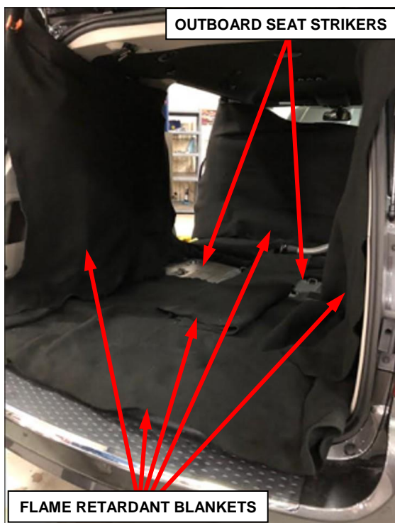
Figure 16 – Protect Interior Surfaces – Leave Outboard Seat Strikers Exposed
