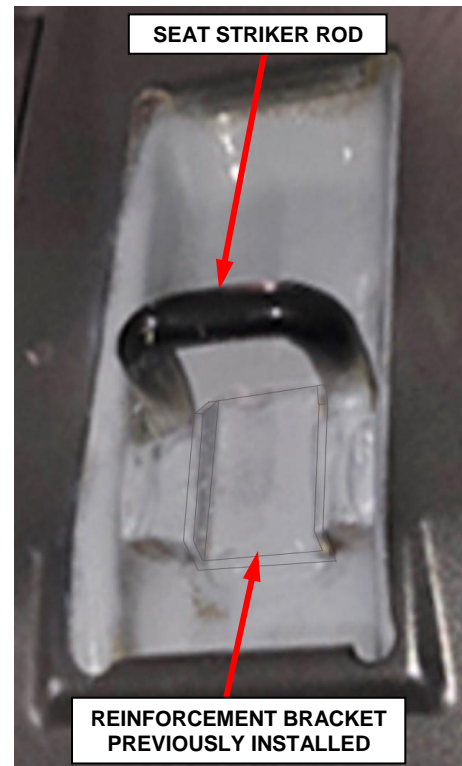
Figure 17 – Reinforcement Bracket Previously Installed
