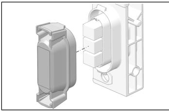
2. Remove the 50A Chassis (top) fuse and discard.
