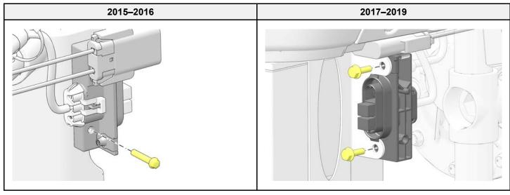
TORQUE Battery Fuse Block Holder Fastener(s): 36 in-lbs (4 N·m)
