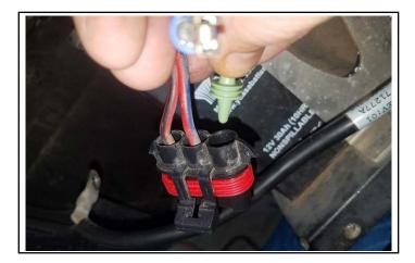
5. Measure roughly ONE inch (1") from the end of the connector. Using a Wire Cutter, snip off the connector end of the red wire that was removed from "Position C" as shown.
