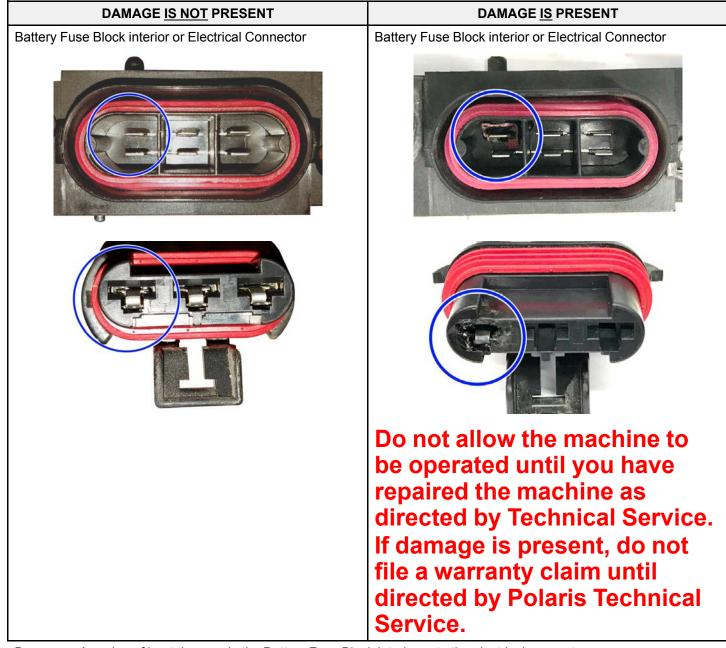
Damage = Any sign of heat damage in the Battery Fuse Block interior or to the electrical connector.
