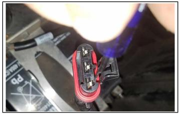
4. Install cavity plug into "Position C" and reinstall the rear secondary locking clip cover to the back of the connector.
