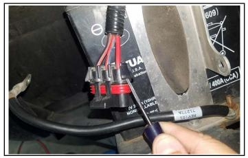
3. Using a pin removal tool, remove the red wire from "Position C" Insert the pin removal tool into the small, round release slot of the associated terminal until it releases the terminal retainer. Gently pull the wire out of the connector.
