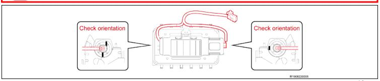
f) Loosely install the plate and airbag inflator with the 2 **NEW** self-locking nuts.
