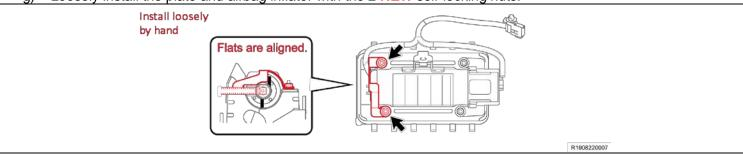
Push the inflator and plate to towards the position determining plate to eliminate any gap.
