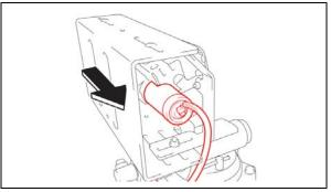
b) Remove the inflator from the airbag assembly and place it on a safe work surface.
