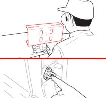
ALWAYS keep as much of your body as possible in front of the bracket when working on the airbag assembly.
