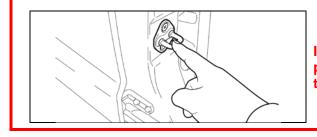
If the anti-static kit is not available, before starting work and periodically while working on the vehicle, touch a metallic part of the vehicle to discharge static electricity in the body.
