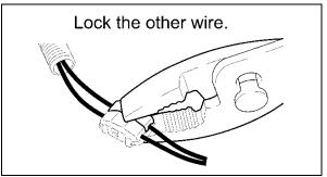
c) Set the other wire in the electro tap and lock it in place using pliers.
