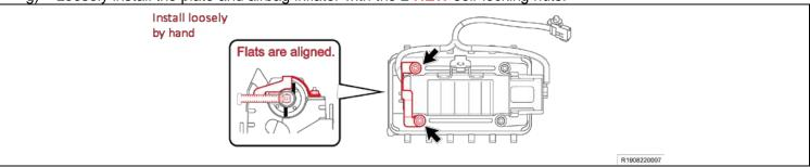
h) Push the inflator and plate to towards the position determining plate to eliminate any gap.
