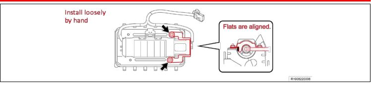
g) Loosely install the plate and airbag inflator with the 2 **NEW** self-locking nuts.
