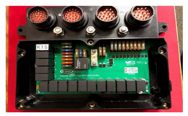
Figure 3 – EIM solid state relay E-One part # 1101384 in K15 position
