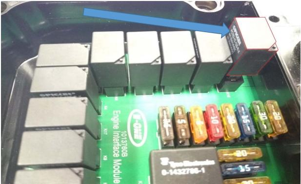
Figure 2 – Remove relay K-15 from far right location
