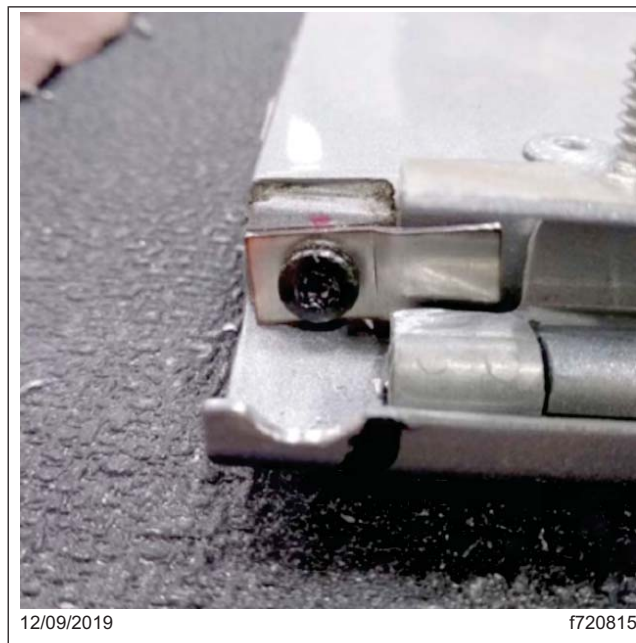
Fig. 5, Installed Hinge Bracket
