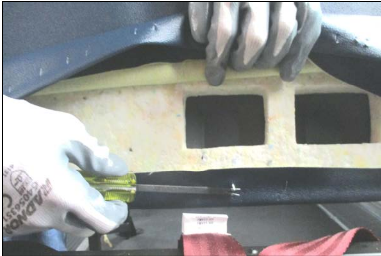
Figure 2: Removing Staples from the Reverse Side of the Vinyl
