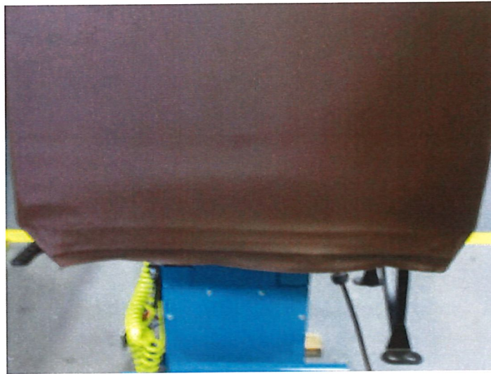
Figure 14: Vinyl shown pulled all the way down (Back of seat)
