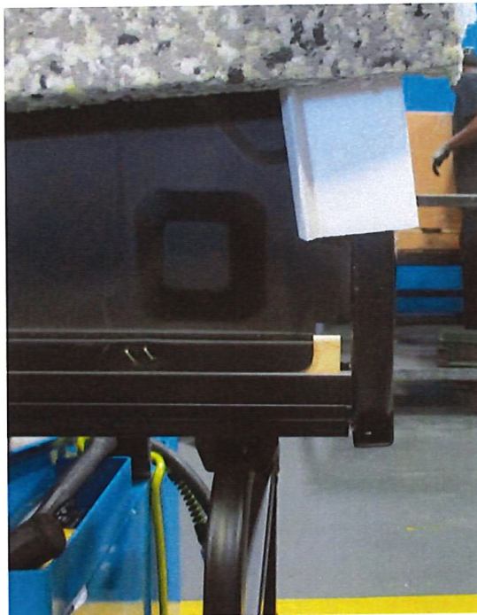
Figure 7: Styrene shown being installed on seat back frame (Right side)
