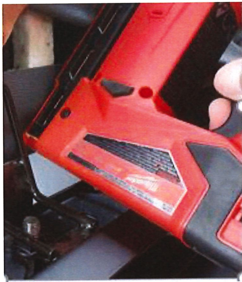
Figure 16: Staple vinyl from back to wooden stick all the way across
