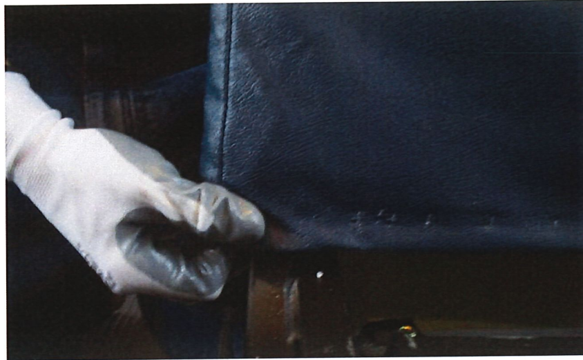
Figure 17: Showing how the Vinyl will look when folded and stapled
