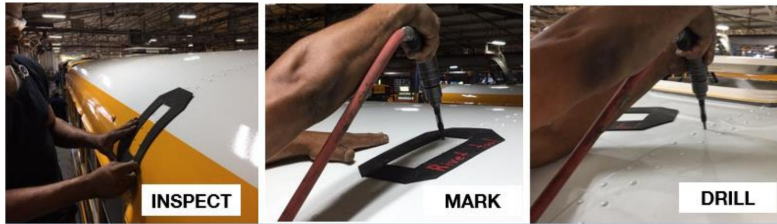
3. Inspect rivet spacing at each roof sheet joint. Roof sheet joints are assembled with two rows of rivets. Joint must have a minimum of six rivets in an eight inch segment. The full length of the roof sheet joint, including the top of the bus, must be inspected and corrected, if needed.
