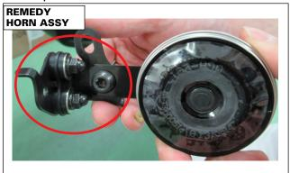
If the original horn assembly (shown below) is currently installed, the repair needs to be performed. Continue to the Recall Repair Procedure section.
