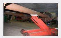
STEP 6: Insert the new bronze bushing (b) into the spring eye. A C-Clamp may be required for this Step.
