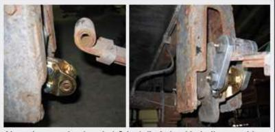
New shear spring bracket & installed shackle bolt assembly.
