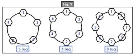
D. Torque wheel lug nuts to the torque values listed in the Wheel Torque Requirement Chart.
