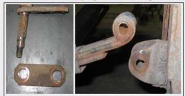
Old shackle assembly and disassembled equalizer.
