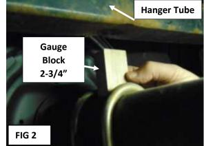
**NOTE:** The gauge block measurement method shown in figure 2 may need repeated after **STEP 3**, and again after **STEP 4** depending on the components changed.
