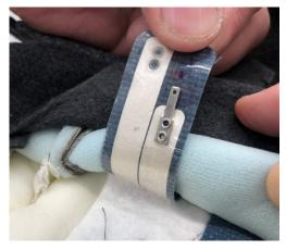
**Step9- IMPORTANT:** Always squeeze the tail terminals firmly at the rivets when disconnecting / reconnecting the harness terminals. Connect the new harness terminals to the sensor mat removing **ONE CONNECTION AT A TIME** to make sure they are reconnected in the proper configuration.
