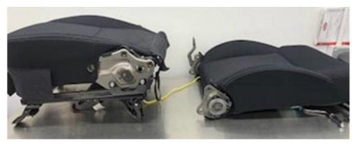
**Step5-** Unclip the two retaining loop / clips from the seat cushion front frame, unhook the elastic loop with a finger and unplug the ODS mat harness from the ODS module as shown in the sequence below.
