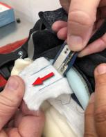
Step8- IMPORTANT: Before connecting the new harness, inspect the tail and sensor mat connectors to confirm they are tight on the 2 metal bands of the mat. Inspect closely for any breaks, cracks or other damage to the visible components of the sensor mat. If any damage is identified, the complete seat cushion assembly must be replaced as the sensor mat is not a serviceable component.
