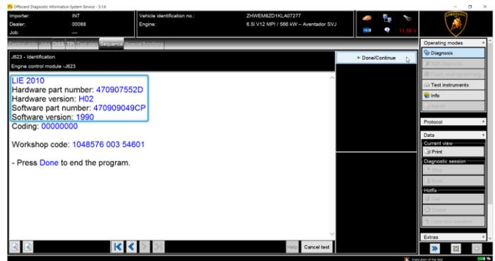
17. Check that Software P.N. and Software version installed are consistent with the "Table of reference for control unit O1" below.
