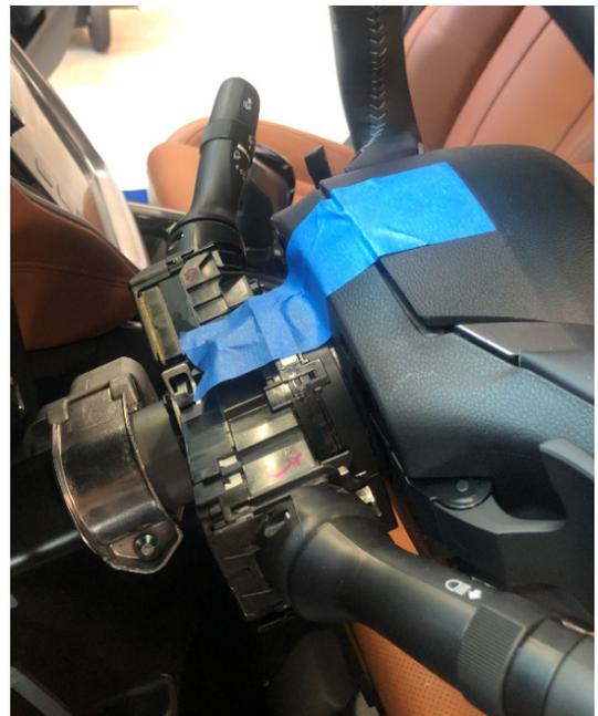
4. Use a piece of wide Painter's Tape or equivalent (tape which will not leave any residue) to keep the steering wheel from turning (and the roll connector in proper position) while the column assembly is removed.
