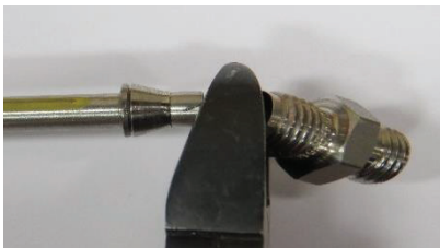
Figure 35: Wire from the LT102B being cut at the pin receiver.
