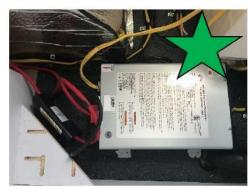
This is correct, the inverter is installed on the floor and the fuse holder is installed on the floor and has the plastic cover installed.
