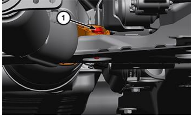
Figure 46 – Front Exhaust Isolator
