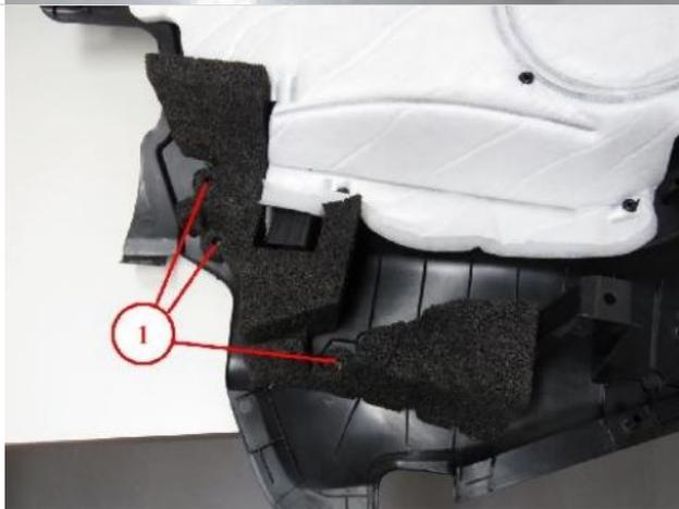
7. Apply adhesive (Hot melt adhesive 3731 P/N 83 19 2 409 987) to the molded foam part.
