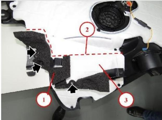
2. Set the molded foam part (1) down and align the existing bore holes over the welded pins (arrows).
