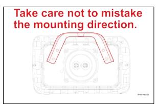
a) Carefully slide the new module into the airbag door.
