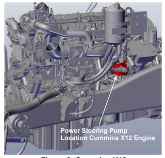
Figure 2, Cummins X12
