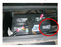
2. Disconnect battery cable from negative post of the chassis battery located under the hood.
