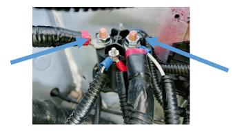
18. Locate and cut yellow ignition power wire, strip back, and connect to yellow wire w/ yellow butt connector from the fuse holder. Crimp and heat shrink using a torch or electric heat gun. Using electrical tape, tape both ends of the yellow wires.
