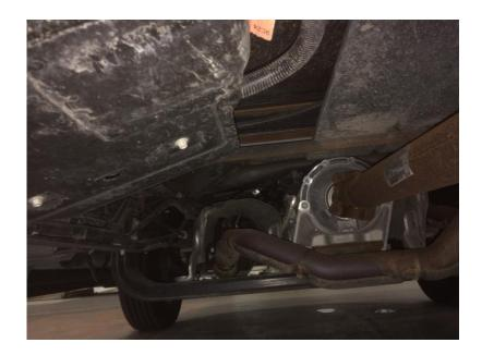
Verify the 2 gauge cable that runs from the Trombetta is supported away from the engine exhaust manifold and the rest of the exhaust, covering the area under the hood to the rear of the cab. If the 2 gauge cable is not secured away from the exhaust manifold or the rest of the exhaust, secure as indicated in the following image.
