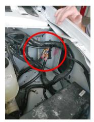
5. Remove the screws holding the BIM/BIR to the inside fender.
