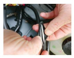
8. Open the loom for the ignition power, locate the yellow wire and cut.
