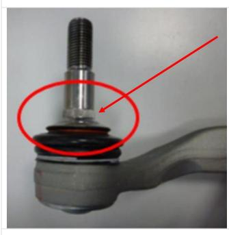
Cone collar disc <u>not</u> installed: knurling visible on the shank (arrow).
