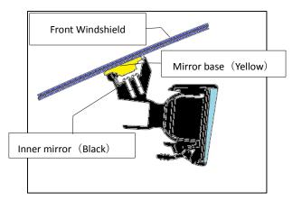
Note: Align the claws of the inner mirror (square in the figure below) with the long three sides (blue) of the six sides of the inner mirror base hexagon. Rotate about 60 degree and fit the claws of the inner mirror with the three short sides (red) of the slit.
