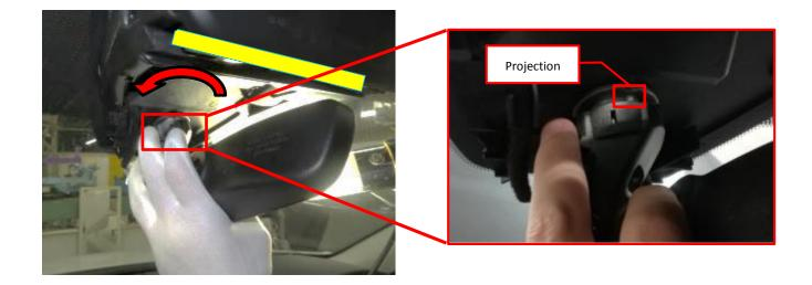
2. Make sure the inner mirror is facing the front and boss is in the red circle position.
