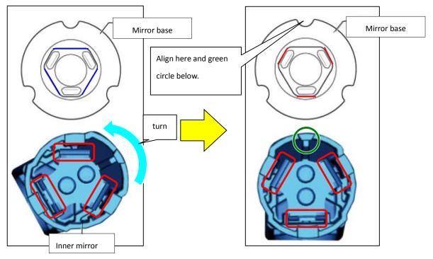
1. Align the projection of the inner mirror at the notch of the mirror base then turn the inner mirror about 60 degree to mount.
