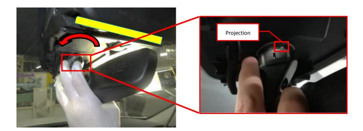
2. Make sure the inner mirror is facing the front and boss is in the red circle position.
