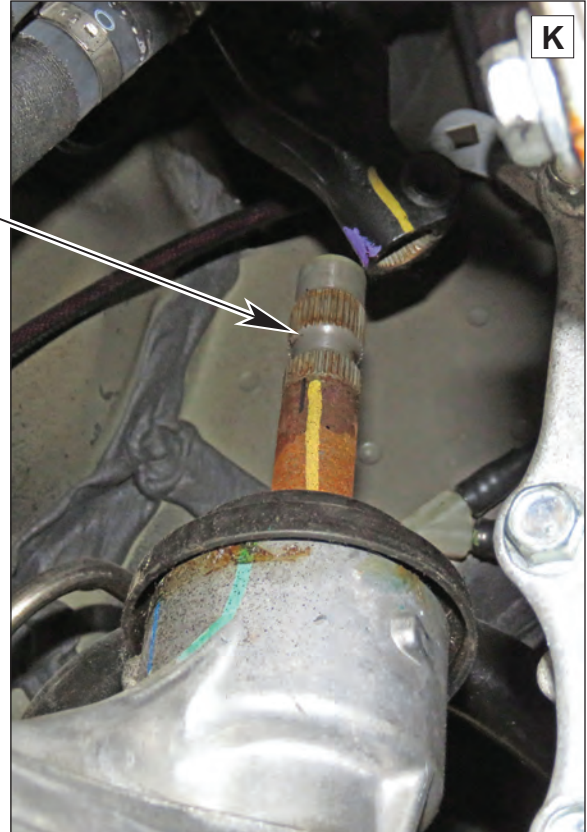
Steering Shaft Extension Removed
