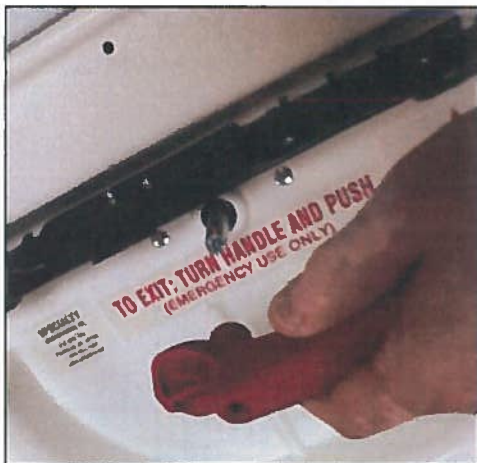
Step 7: Pull down to remove the red handle
