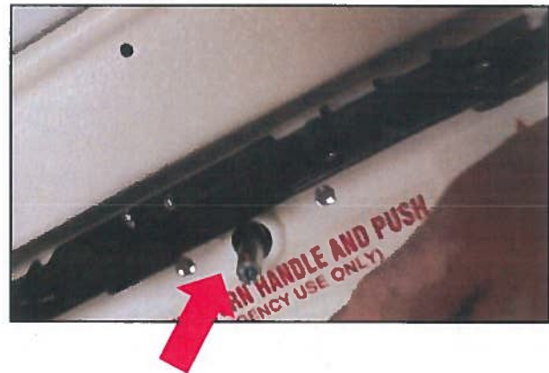
Step 12: From inside the lid, you will see the shaft of the outer handle
