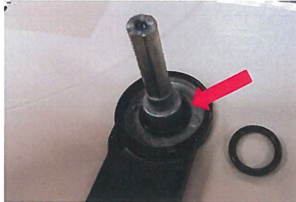
Step 10: Ensure that the 009321-5 O-ring is secured around the base of the handle stem. If it is not there, check to see if it is in the lid bushing. If it is not in either location, replace with a new o-ring.
