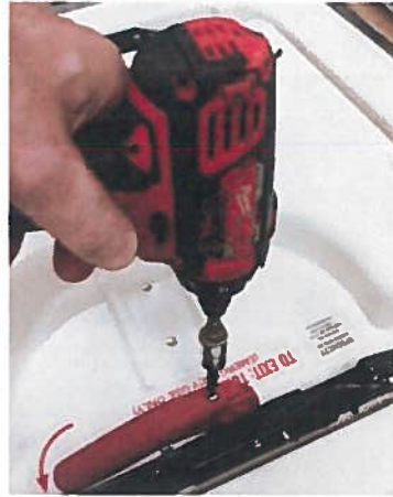
Step 6: Insert the 1/8" Allen bit into the 008798 screw and remove screw from red handle.
