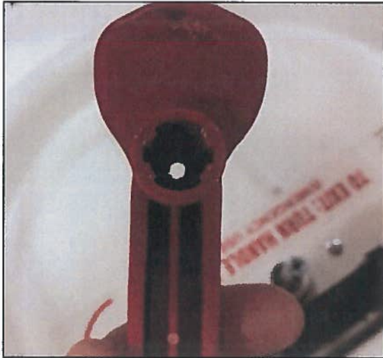
Step 13: The inside of the red handle has ribs to self-orient the red handle on the outer handle.
