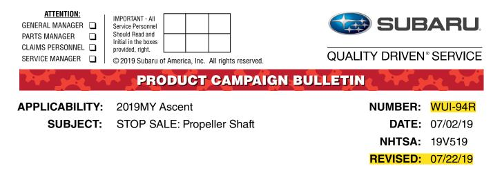
Subaru of America, Inc. (Subaru) is recalling certain 2019 model year Ascent vehicles, due to a potential propeller shaft carrier mounting bolt tightening torque issue. A total of 166 U.S. vehicles will be affected by this recall. The repair will involve replacing the propeller shaft and related bolts in all potentially affected vehicles.
