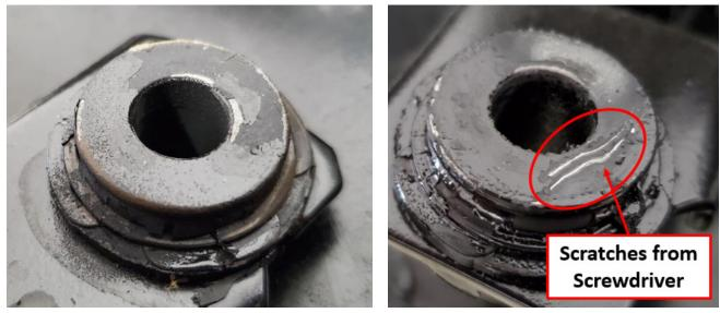
These **OK** photos show the body side of replacement parts with a much lighter, uniform coating.
