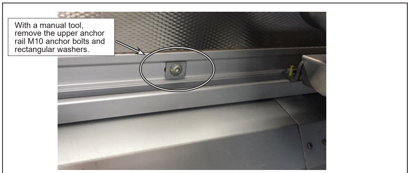
Figure 12 - M10 Bolts and Rectangular Washers to Remove
