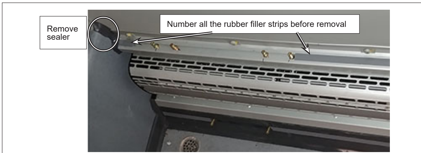
Figure 11 - Typical Anchor Rail, Rubber Filler Strips and Sealer
