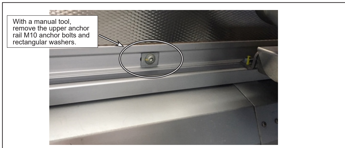
Figure 12 - M10 Bolts and Rectangular Washers to Remove
