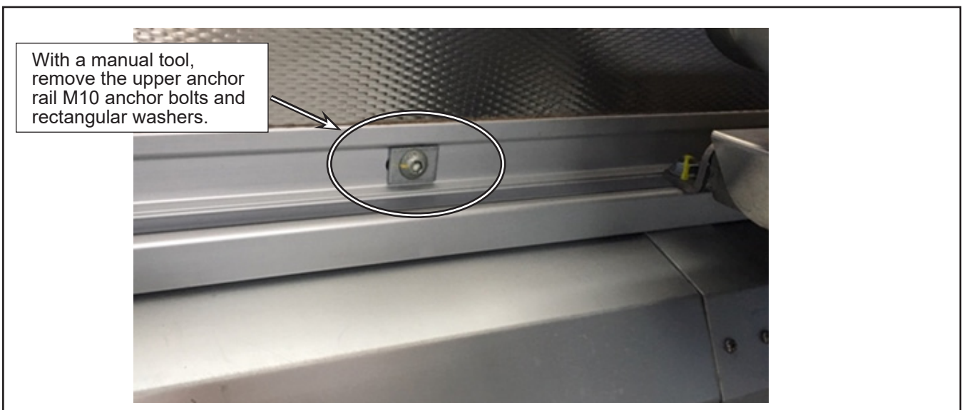
Figure 12 - M10 Bolts and Rectangular Washers to Remove
