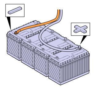
11. Connect the cable to the negative terminal.
