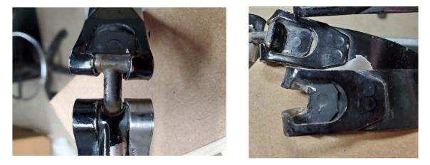
If the inspection shows a failed strap, continue with the repair procedure.
