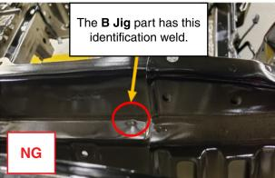
7. If the cowl area inspection reveals an A JIG part, the vehicle is OK. STOP, take a clear photo of this area and the VIN plate at the base of the "B" pillar. Reinstall all the removed parts in reverse order to prepare the vehicle for sale. Proceed to Step 8.
