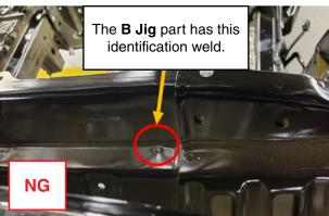
7. If the cowl area inspection reveals an A JIG part, the vehicle is OK. STOP, take a clear photo of this area and the VIN plate at the base of the "B" pillar. Reinstall all the removed parts in reverse order to prepare the vehicle for sale. Proceed to Step 8.
