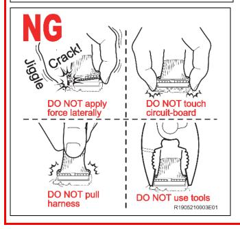
DO NOT disconnect the flat cable of the MG-ECU (the upper side with the PEN sheet) since it may be broken. Make sure to disconnect the IPM side (the lower side).
