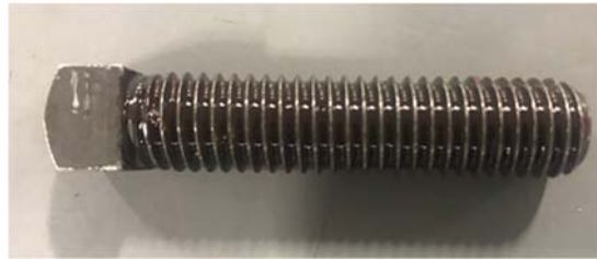
Figure 11 – Loctite® 263 on Stop Bolt Threads
