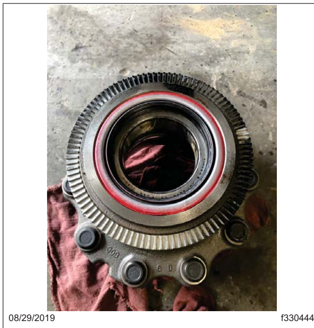
Fig. 25, Joint de moyeu installé
