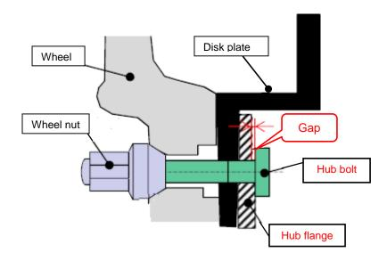
The repair is to retighten the front and rear wheel lug nuts from 137 Nm (101 ft. lb.) to 147 Nm (108 ft. lb.).
