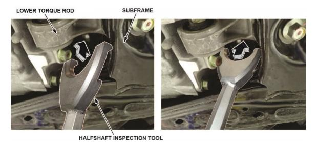
6. Place the open face against the inboard joint of the driveshaft. Make sure the curved edge of the tool is flush with the inboard joint as shown.
