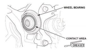
15. Install the outboard joint into the hub assembly.
