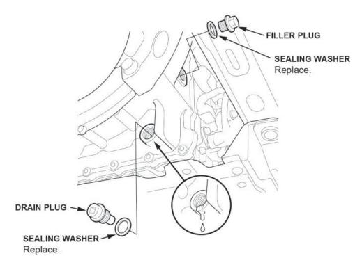
3. Remove the drain plug with the sealing washer, and drain the ATF until it slows to a slight drip.
