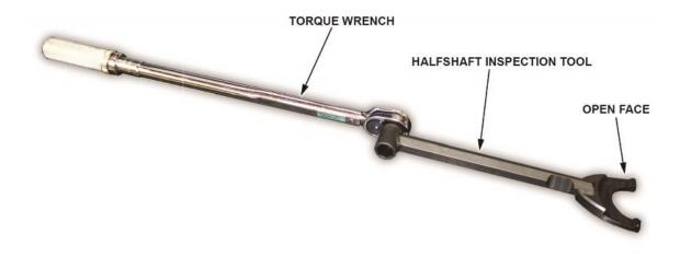
5. Keep the tool lined up with the torque wrench. Insert the tool through the gap between the lower torque rod bracket and the subframe. Turn the tool until the open face is toward the right of the vehicle.
