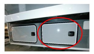
2. Once inside compartment, locate box on left hand side and remove box cover.
