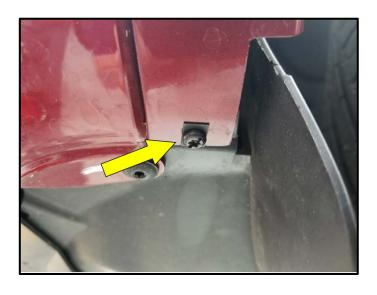
Install securing fasteners on both front and both rear wheel arch covers.
