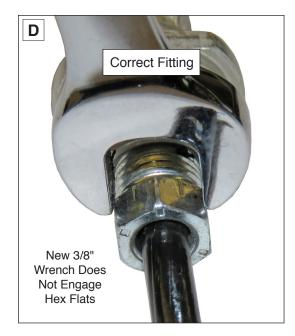
Place new 3/8" wrench onto brake line fitting shown in Photo B. If wrench **does not** engage hex flats, the correct line fitting is installed. See Photo D. If the new 3/8" wrench **does** engage hex flats the brake line adapter fitting (included in kit) must be installed. See Photo E.
