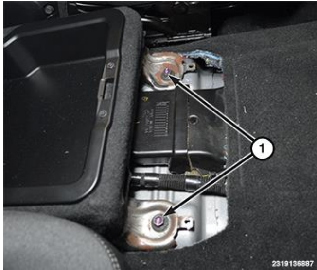
Figure 9 – Center Seat Front Fasteners
