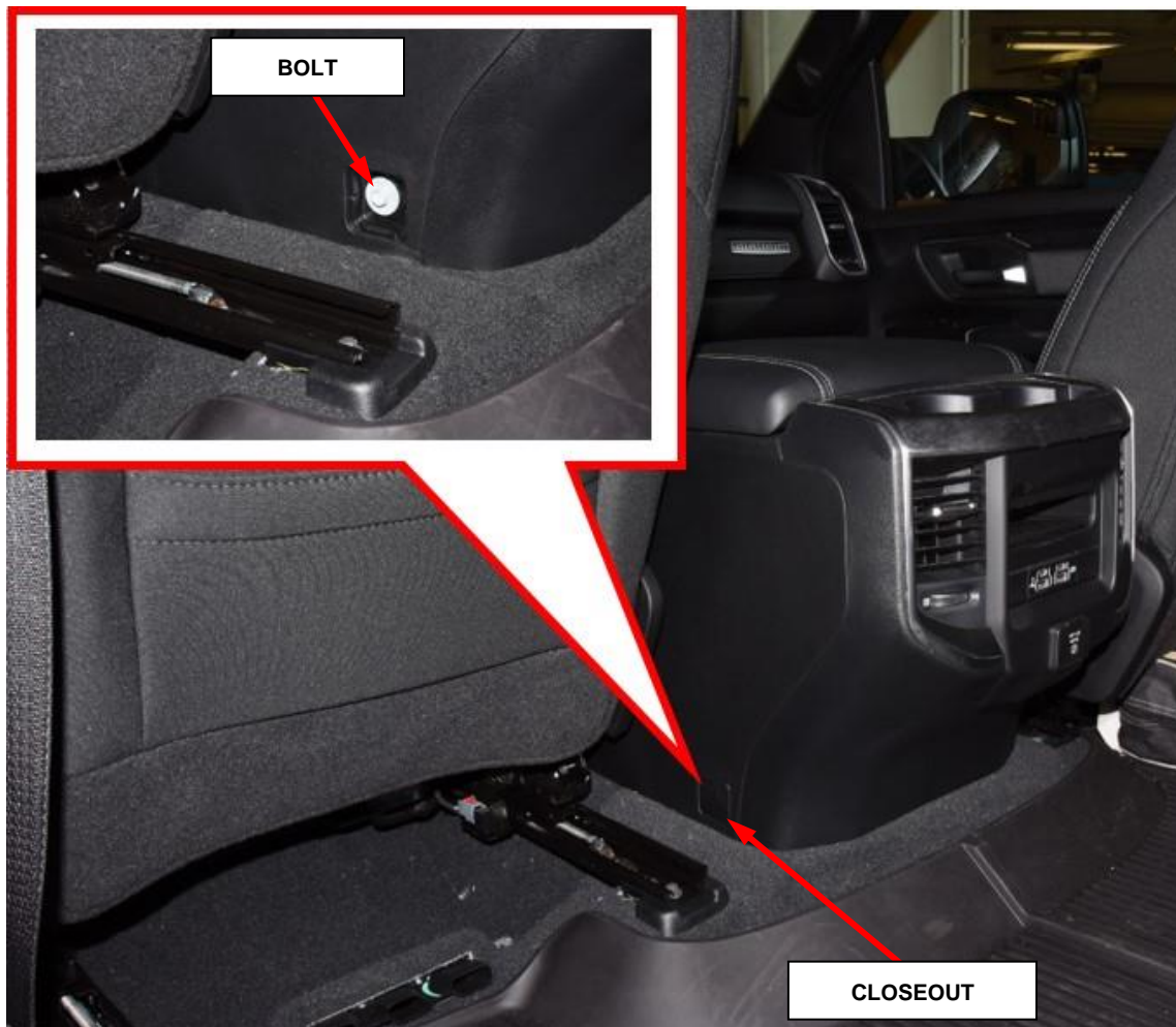
Figure 1 – Floor Console Closeouts and Fasteners Rear
