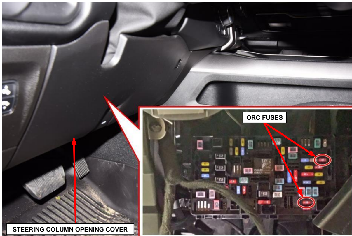
Figure 16 – ORC Fuses F28 and F65
